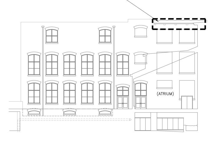
Contractor to remove loose, flaking, peeling, and cracked exterior LBP from the roof beams (rafter tails, soffit, and facia down to stable paint layer. Where wood is found to be damaged, Contractor to consult with GC and Owner's Representative as to the limits of removal. Where wood is removed, Contractor to temporarily seal areas open to the interior of the Building to protect interior surfaces from damage and exposure to the elements.
